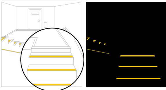
and shall extend for the full length of the step. Outlining stripes shall have a minimum horizontal width of 1 inch (25 mm) and a maximum width of 2 inches (51 mm). The leading edge of the stripe shall be placed at a maximum of 1/2 inch (12.7 mm) from the leading edge of the step and the stripe shall overlap the leading edge of the step by not more than 1/2 inch (12.7 mm) down the vertical face of the step.
