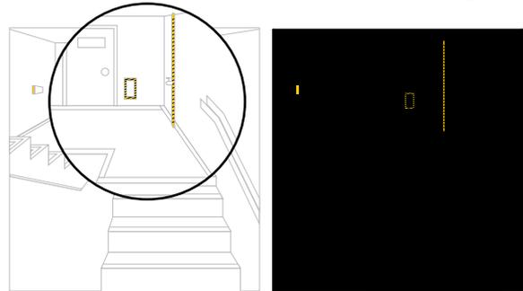
equal bands, of luminescent luminous material and black, with the alternating bands no more than 2 inches (51 mm) thick and angled at 45 degrees (0.79 rad). Obstacles shall include, but are not limited to, standpipes, hose cabinets, wall projections and restricted height areas. However, such markings shall not conceal any required information or indicators including, but not limited to, instructions to occupants for the use of standpipes.
