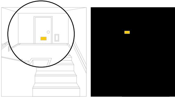
NFPA 170. The exit symbol shall be a minimum of 4 inches (102 mm) in height and shall be mounted on the door, centered horizontally, with the top of the symbol no higher than 18 inches (457 mm) above the finished floor.
