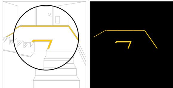
The leading edge of landings shall be marked with a stripe consistent with the dimensional requirements for steps.
